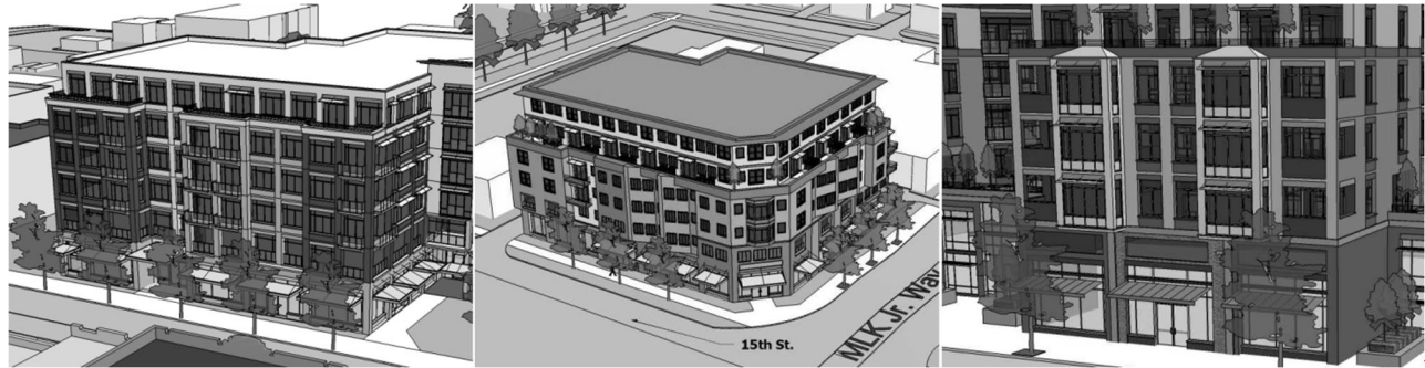
Below: Articulation examples of mixed-use buildings containing residential uses on upper floors. These examples include vertical and horizontal modulation and changes in building materials at no more than 30-foot articulation intervals.
