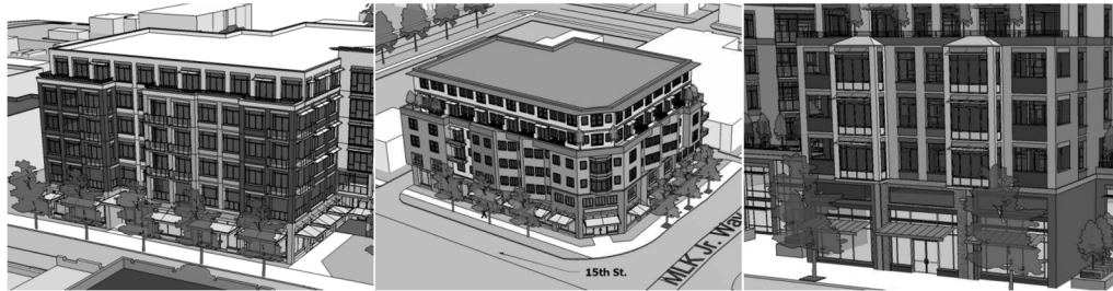
Articulation examples of mixed-use buildings containing residential uses on upper floors. These examples include vertical and horizontal modulation and changes in building materials at no more than 30-foot articulation intervals.
