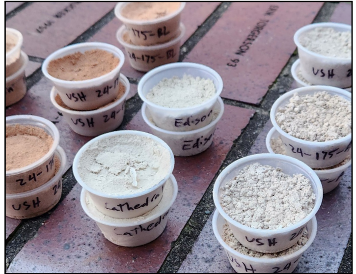
Mortar samples on-site prior to being cleaned and rinsed concurrent with the masonry. Two samples were prepared for each mortar type; only one sample was cleaned.
