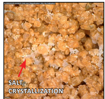
B3.3 - USHG (DARK) Salt crystals visible in many areas of the sample. Translucent characteristics of the aggregate
