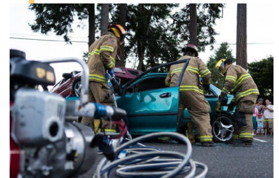
Tacoma Fire Department demonstrates an emergency passenger extraction using the 'jaws of life'
