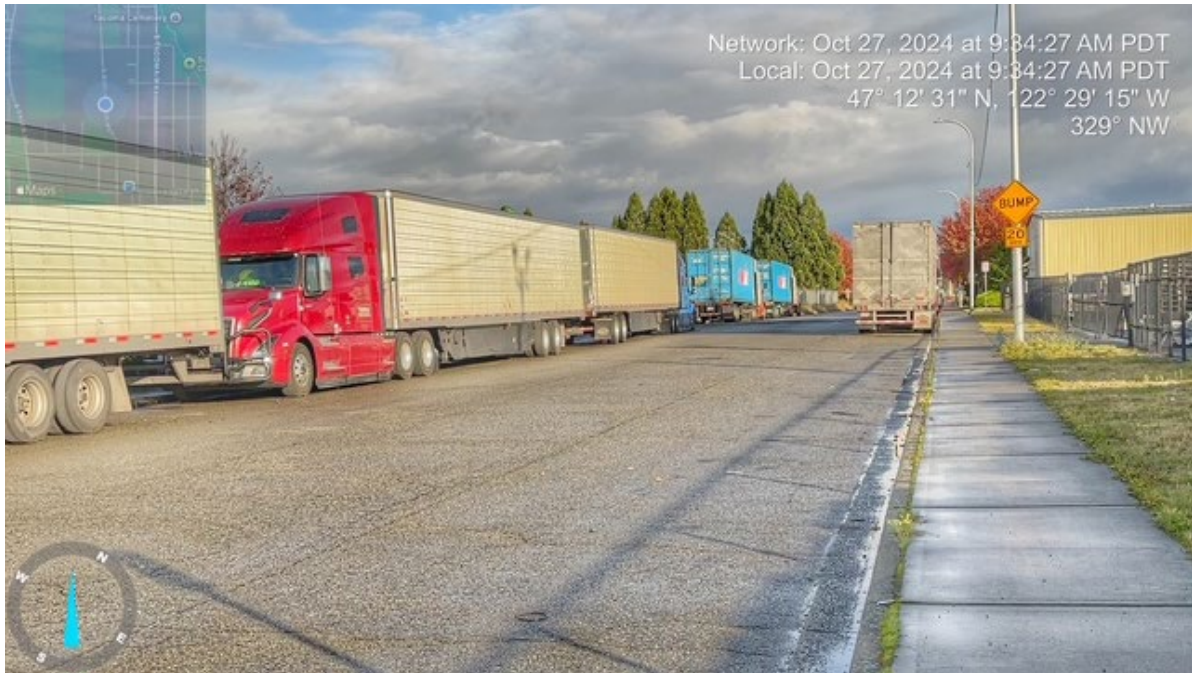
Here the sidewalk on the East side of the street is narrowed to five feet even though there is room for a 7 foot walk.
