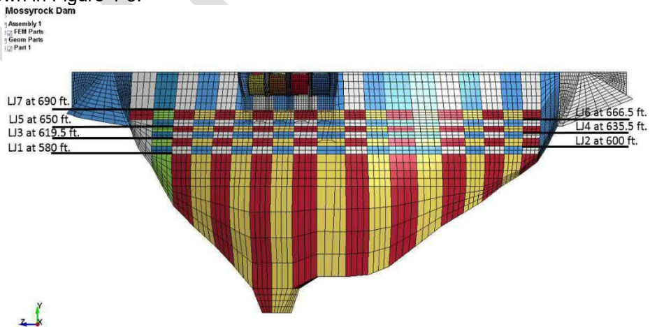
Figure 4-2: Lift Line Elevations
