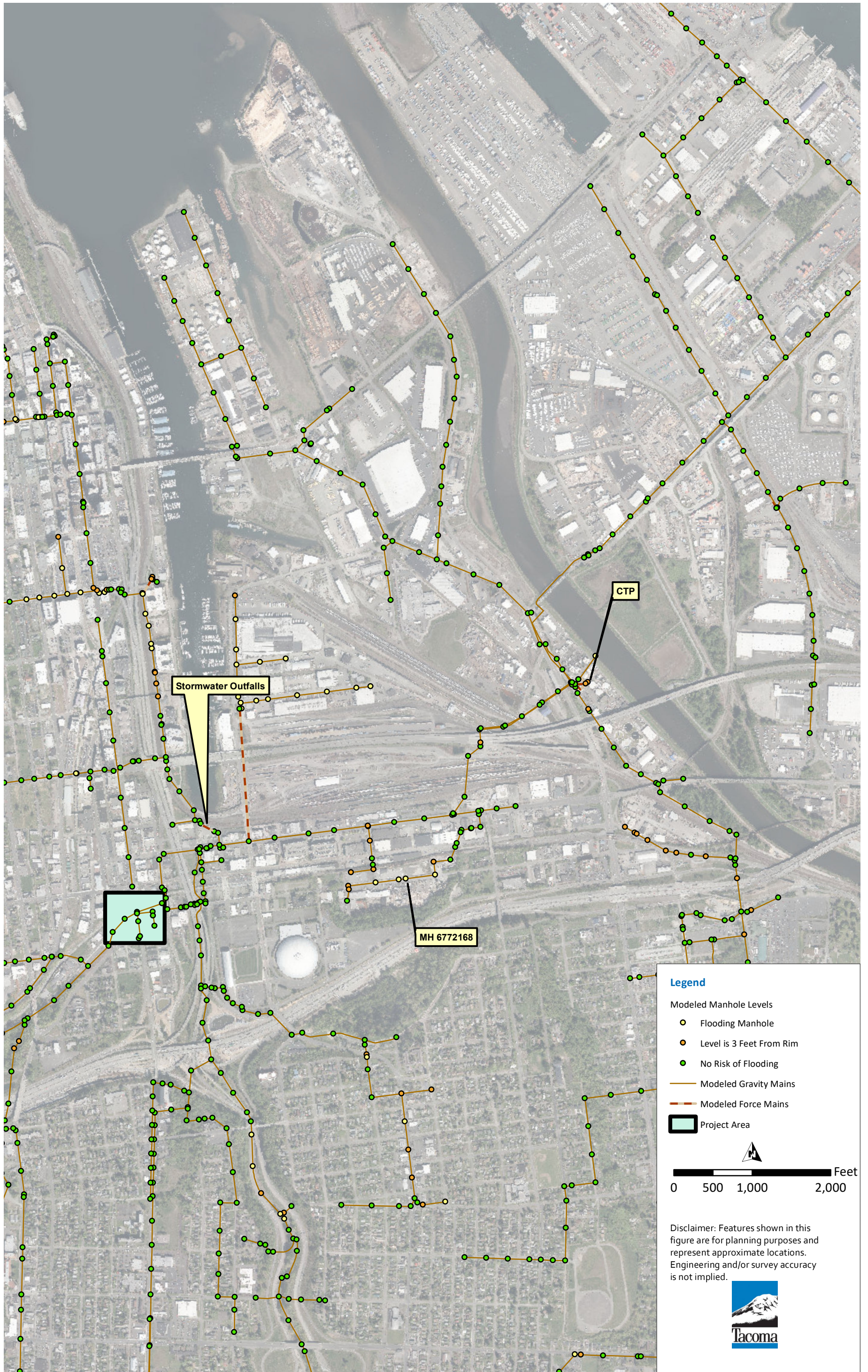
Figure 9 Proposed Sanitary Sewer Alignment Deficiencies for Design Storm at Buildout Flows
