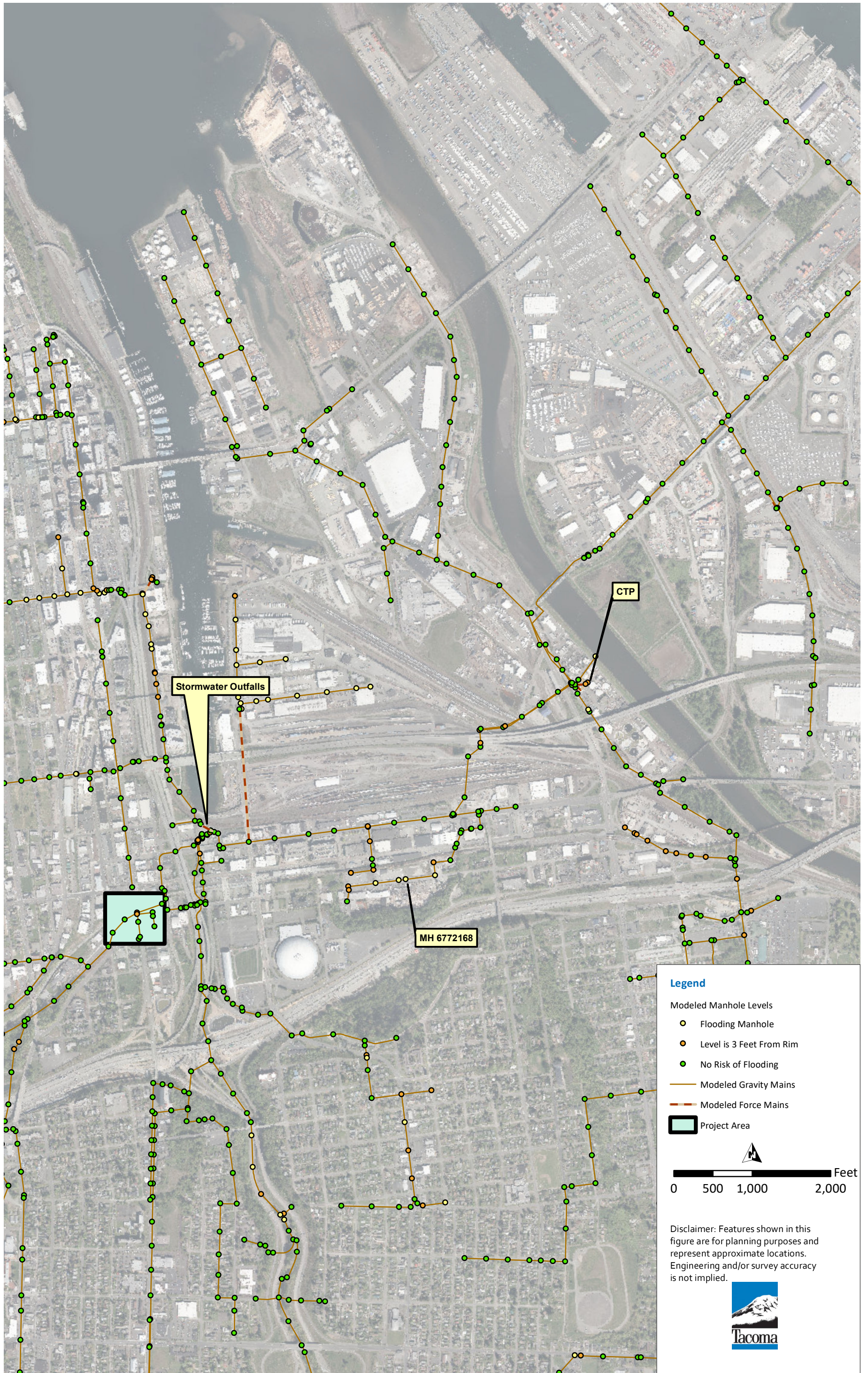
Figure 8 Current Sanitary Sewer Alignment Deficiencies for Design Storm at Buildout Flows
