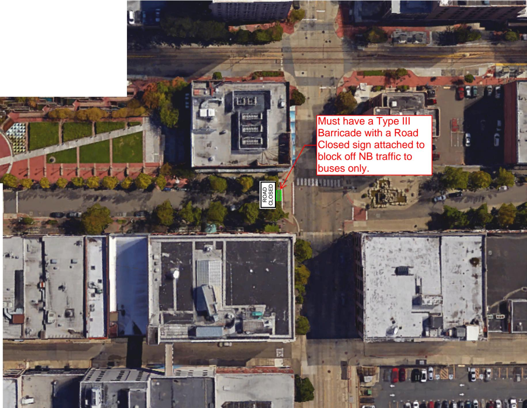
Must have a Type III Barricade with a Road Closed sign attached to block off NB traffic to buses only.
