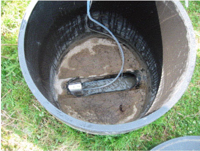
Figure 7-5c Flow Monitoring setup for Pervious Pavement and Standard Asphalt Sites
