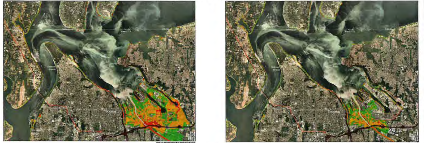
Modeled Inundation from a Tacoma Fault (left) and a Tacoma-Rosedale Fault (right) Tsunami
