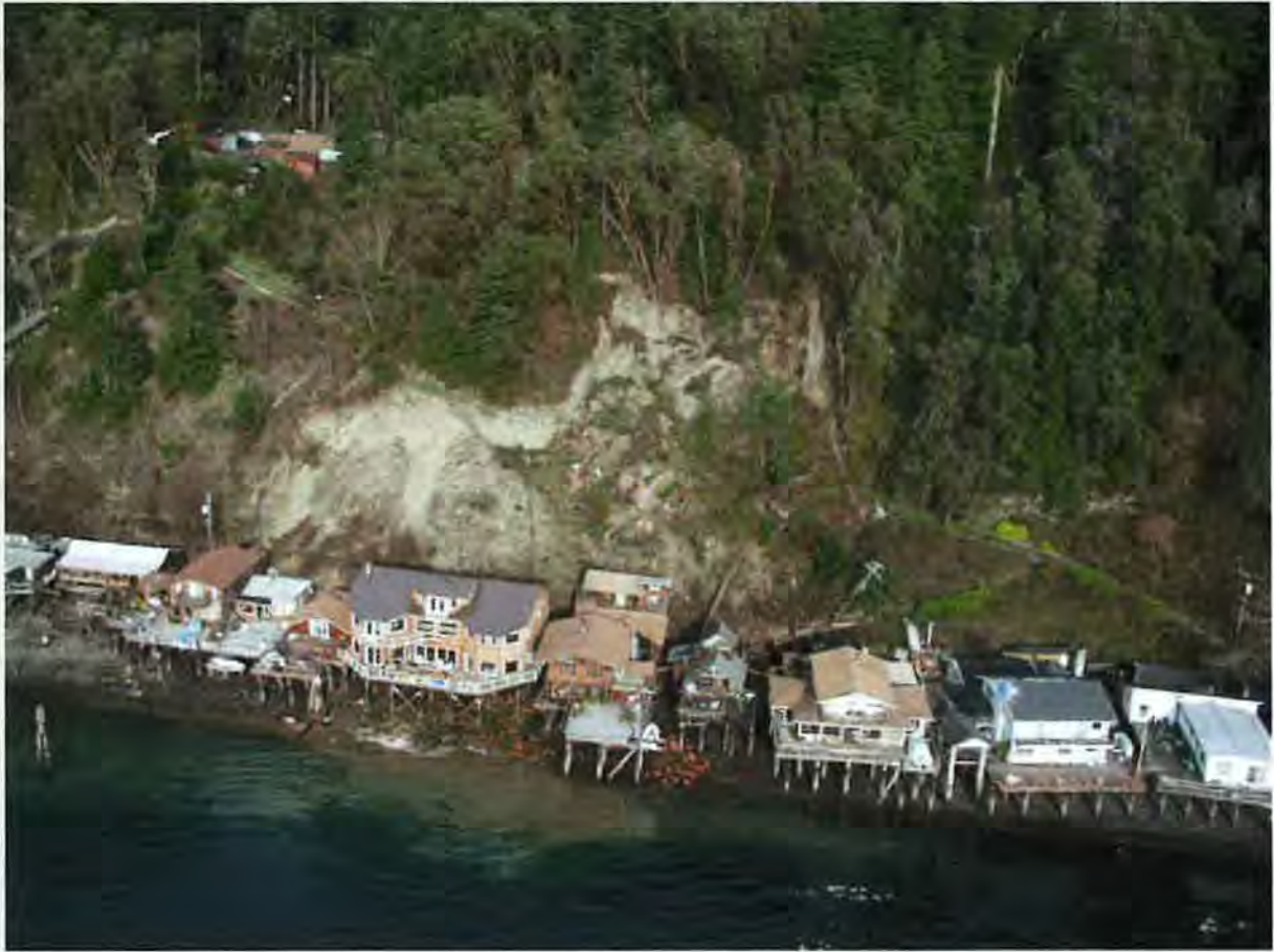
Earthquake shaking may cause landslides on slopes, particularly where the ground is water saturated or has been modified (for example, by having stabilizing vegetation removed). This photograph shows landslides at Salmon Beach, near Tacoma, that were caused by the 2001 magnitude 6.8 Nisqually earthquake, which resulted in an estimated $2 billion in damage and is one of the largest recorded quakes in Washington's history. Slopes along coastal areas of the southern Puget Sound region are particularly vulnerable to landsliding during powerful earthquakes.
